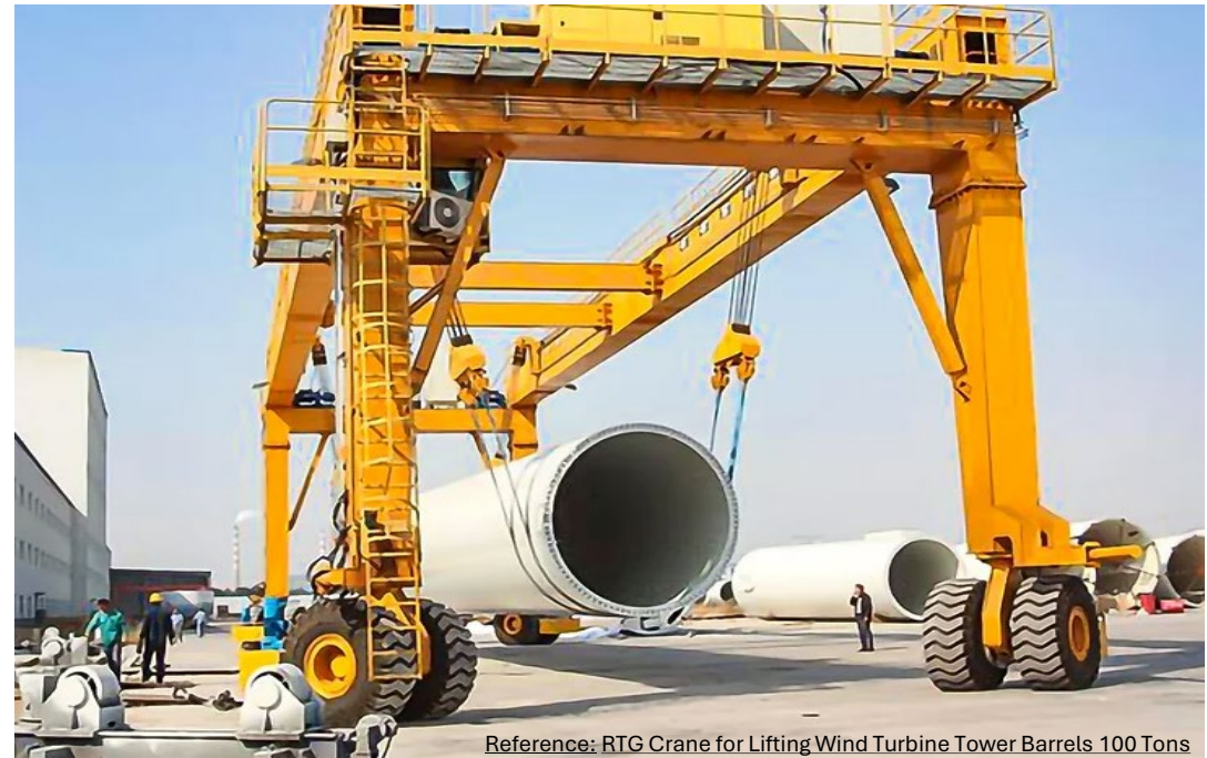
Reference: RTG Crane for Lifting Wind Turbine Tower Barrels 100 Tons
