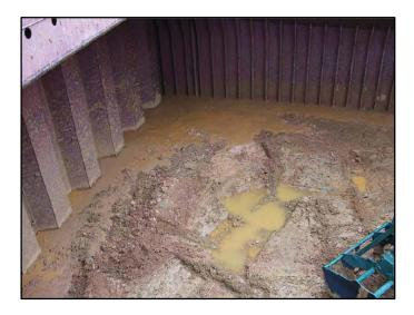
If the propensity for liquefaction is missed during loading and/or prior to departure, a sudden list can easily develop as cargo in the holds liquefies and suddenly shifts en route assisted by the vibration of the vessels engine and movement at sea.
